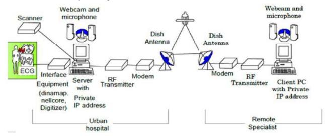
Figure 7. Point to point connection using VSAT (Onuh et al., 2019)
