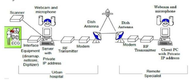
Figure 8: Point to multipoint connection using VSAT (Onuh Spencer Ojogba et al, 2019)
