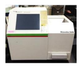
Figure 1. NIR spectrometer, model BR-5000
