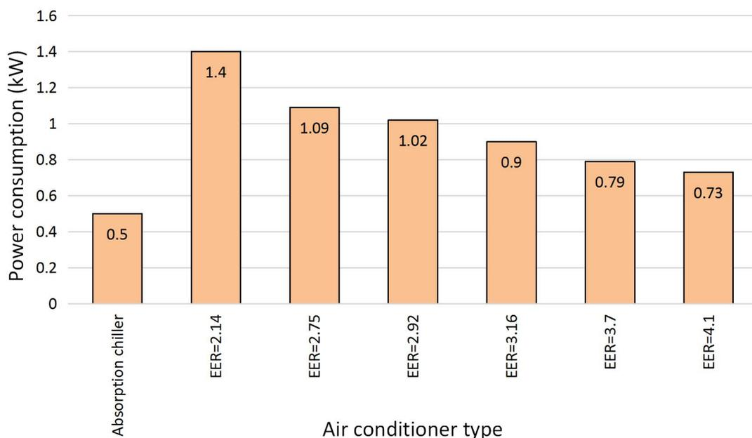
Figure 6: Comparison of power consumption by the absorption cooling system with that consumed by conventional vapour compression chiller of varying EER
