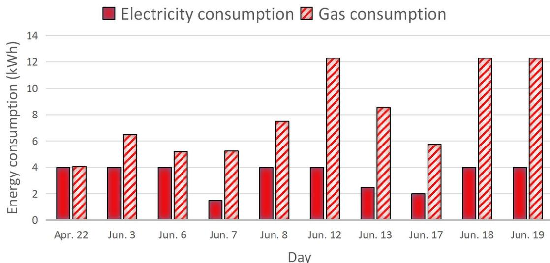
Figure 4: Energy consumption of the absorption chiller for the experimental days
