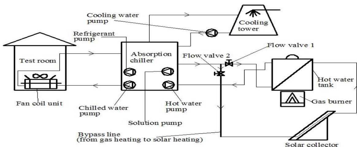
Figure 1: Schematic of the experimental set up
