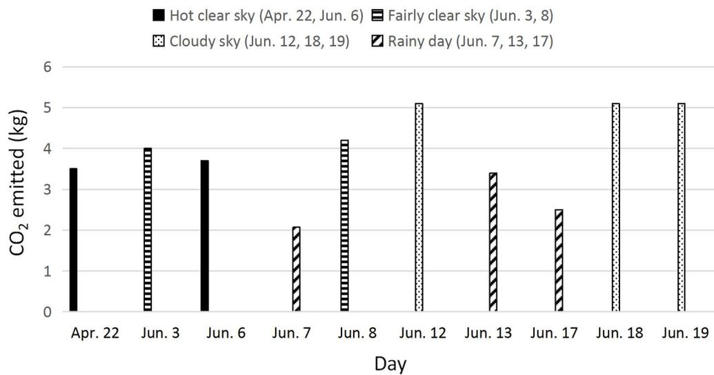
Figure 5: CO<sub>2</sub> emitted by the absorption cooling system for the experimental days.
