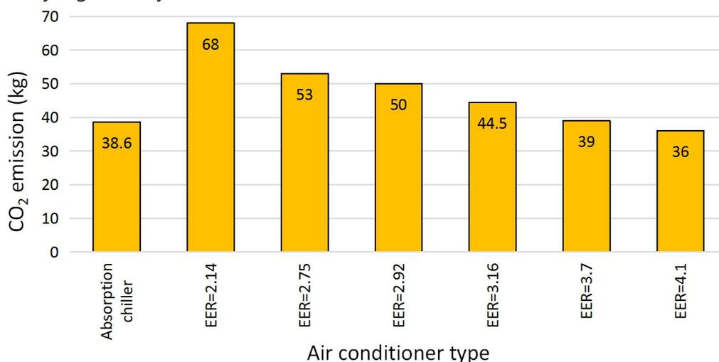
Figure 7: Comparison of CO<sub>2</sub> emission by absorption cooling system to CO<sub>2</sub> emission by conventional chiller of varying EERs
