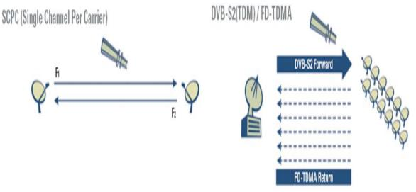
Figure 10: SCPC vs. TDMA (Maral et al., 2011)
