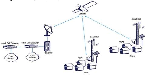
Figure 14: Gilat's Cell-Edge over Satellite Solution (Source: Doreet, 2014)
