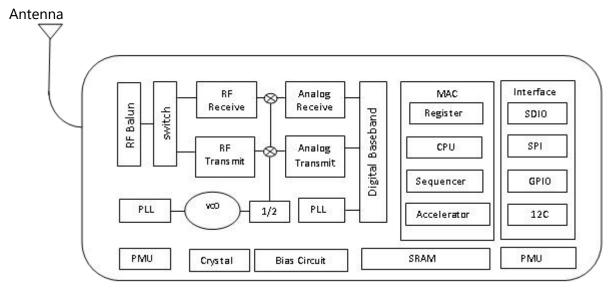
Figure 1: Description of the ESP8266 module
