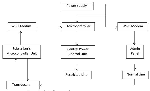
Figure 2: Block diagram of the power management system
