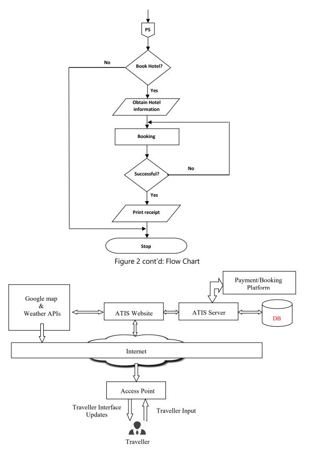
Figure 3: System architecture
