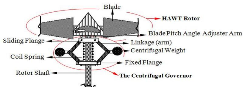
Figure 2: Centrifugal Governor on the HAWT rotor shaft
