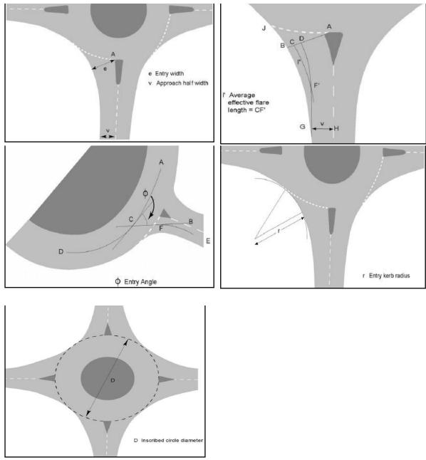
Figure 1: Definition of Roundabout Features (DMRB, 2007)
