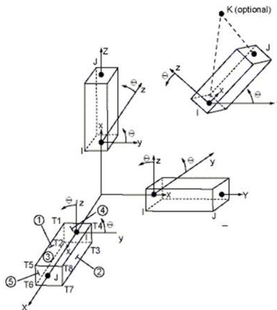
Figure 7: Details of the Beam 4 3D geometry adapted from the ANSYS material library
