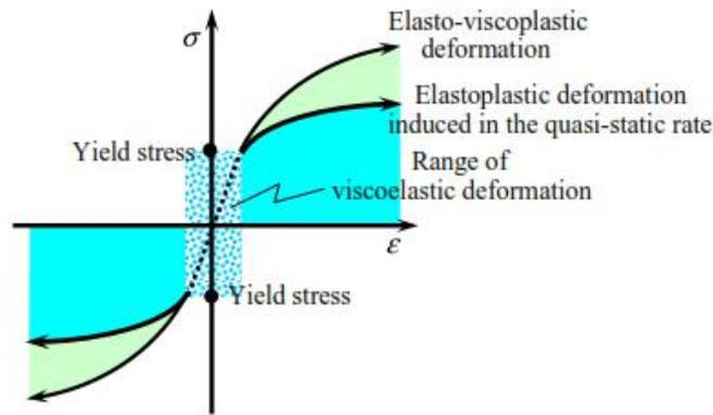
Figure 3: Rate dependent deformation of solids adapted from Hashiguchi, (2014)
