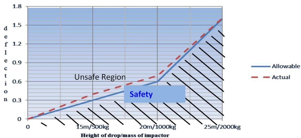
Figure 10: A graph of actual versus allowable displacement considering the effects of other loads for quarter span deflection adapted from Aliyu, (2019)
