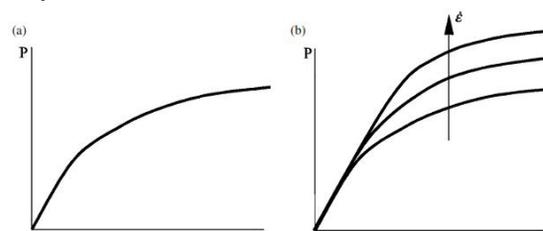
Figure 1: Engineering stress-strain curve a) rate-independent b) rate-dependent adapted from Belytschko et al. 2014.
