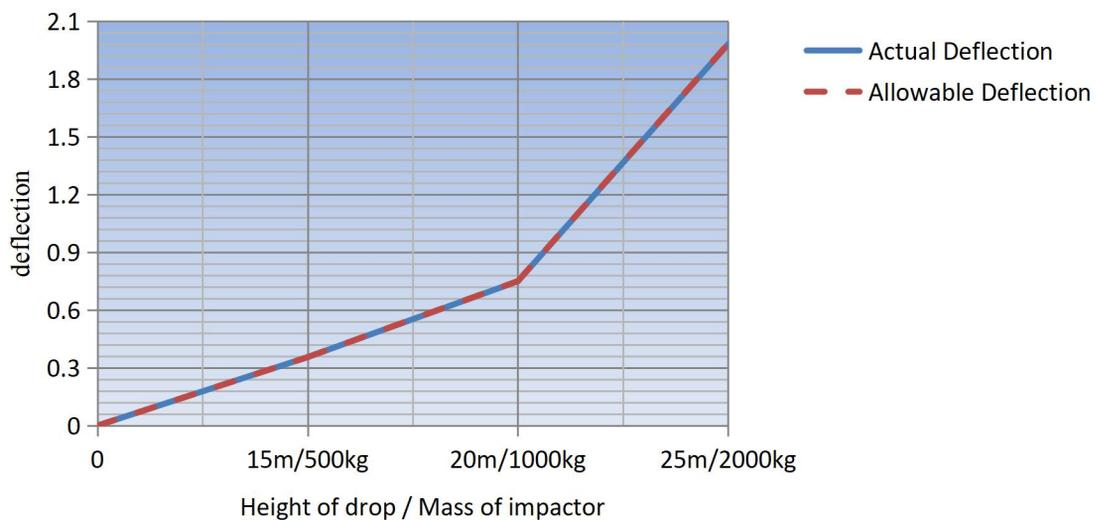
Figure 9: A plot of actual versus allowable displacement considering the effects of other loads for mid span deflection adapted from Aliyu, (2019)
