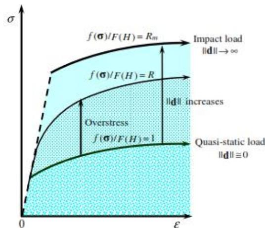
Figure 5: stress-strain cure predicted by the modified overstress model adapted from Hashiguchi, (2014)
