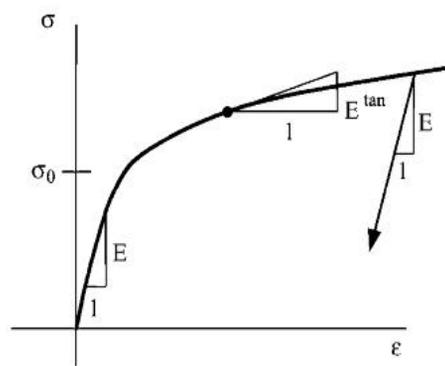
Figure 2: Stress-strain curve for a typical elastic–plastic material adapted from Belytschko et al. (2014)
