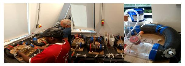
Figure 6. Arrays of the 12 litres innertube digesters been tested
