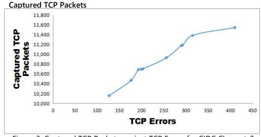
Figure 3: Captured TCP Packets against TCP Errors for CIDC Claranet\_2
