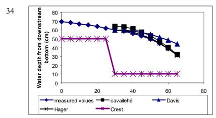
Figure 3: Graph of comparison between the three equations and measurement at 60 l/s
