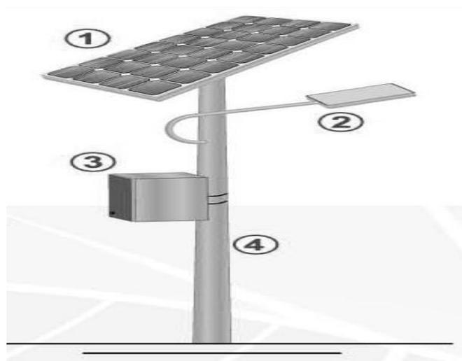
Figure 1: Schematic diagram of a solar powered streetlight
