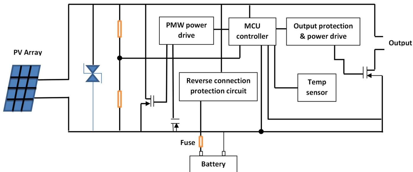
Figure 3: Block diagram of a controller
