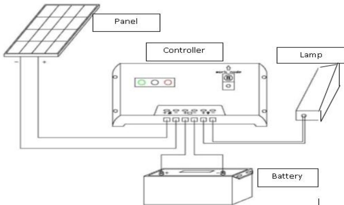
Figure 4: Installation diagram of the solar powered streetlight
