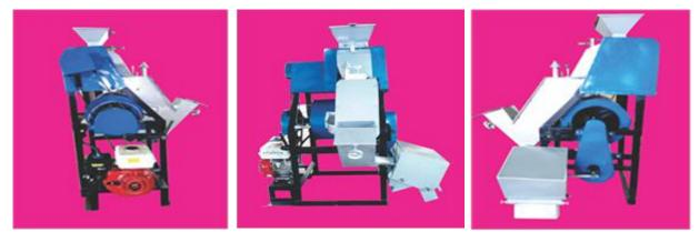
(a)Left end view (b) Front view (c) Right end view Figure 1: Melon Seeds Shelling and Separation Machine
