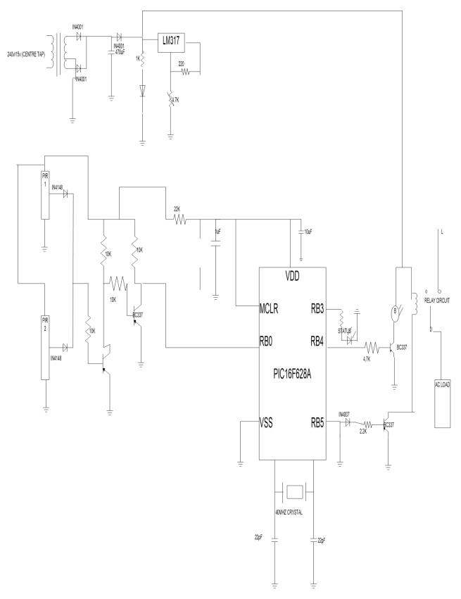
Figure 3: The complete circuit of a switching system using a PIR
