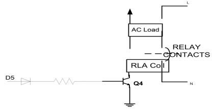
Figure 9: Relay interface circuit
