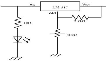
Figure 8: Voltage regulator circuit
