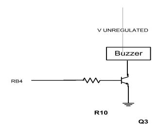
Figure 10: Buzzer interface circuit
