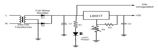
Figure 5: Power supply circuit
