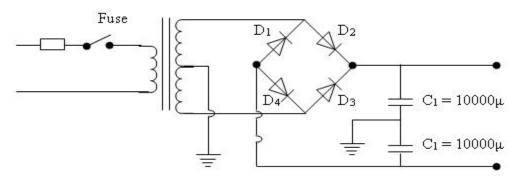
Figure 7: Power Supply Unit
