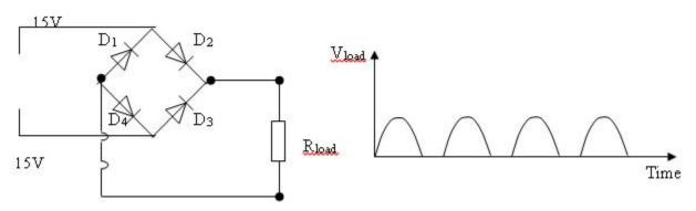
Figure 6: Circuit for Rectification and the Output Waveform
