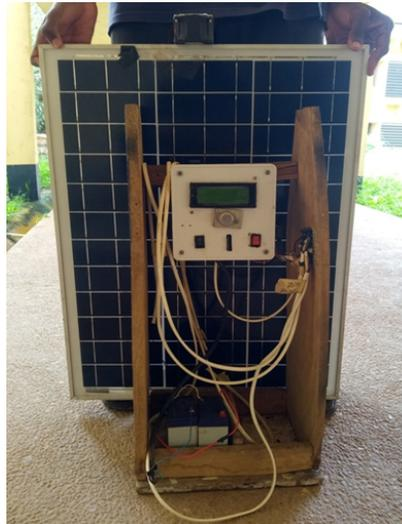
Figure 2: Experimental setup of the onboard controller and solar panel
