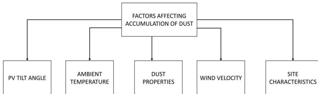
Figure 1: Factors affecting the accumulation of dust on solar panels (Mani and Pillai, 2011)
