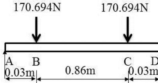
Figure 1: Loadings on the central shaft of drum
