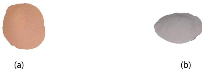
Figure 2: (a) Laterite soil sample. (b) Eggshell powder
