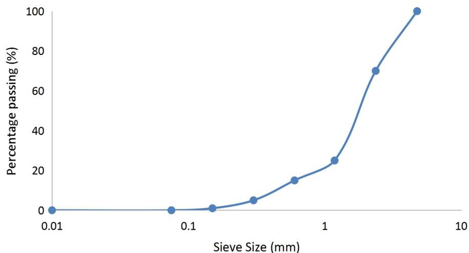
Figure 1: Sieve analysis result for crushed bone.
