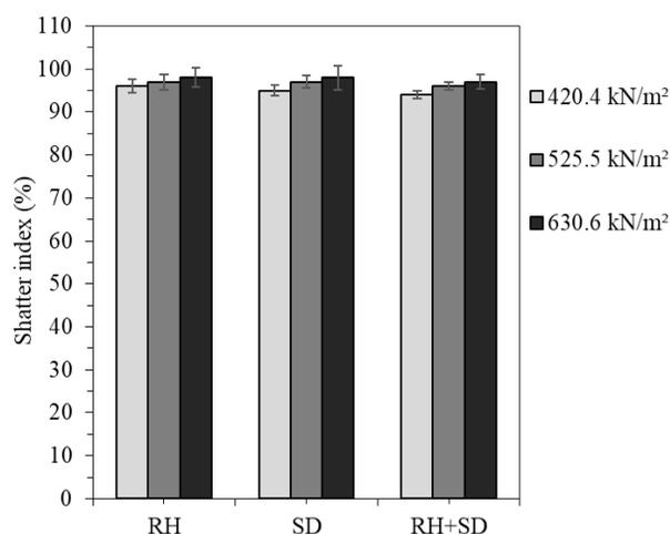
**Figure 6:** The shatter index of the produced briquettes
