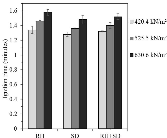
**Figure 9:** Ignition time of the produced briquettes
