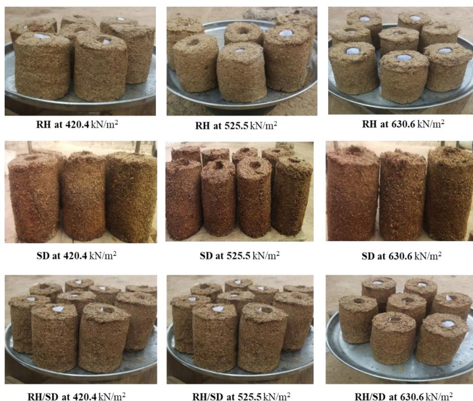
**Figure 3:** The produced briquettes at the different compaction pressures
