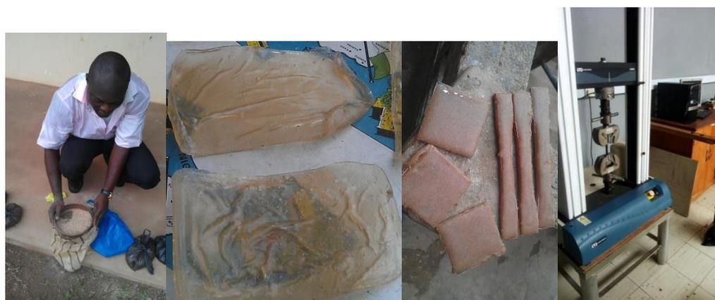
Figure 1: (a) sieving of sawdust, (b) bioplastic, (c) test sample, (d) tensile test on machine
