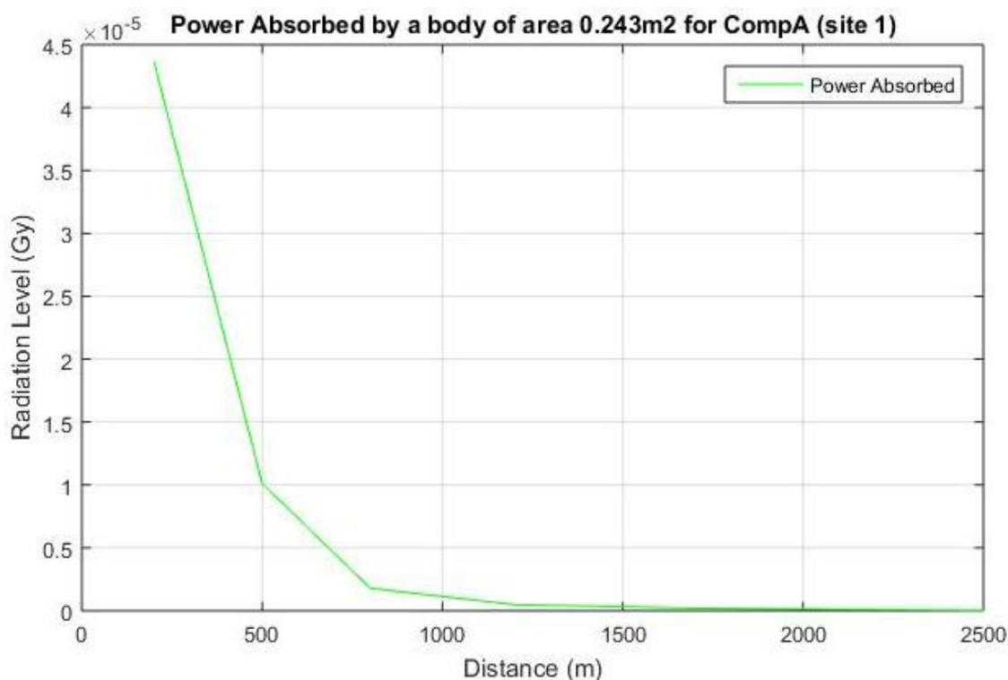
**Figure 1:** Radiation power level against distance by a body with area of 0.243m<sup>2</sup> from COMPA (site 1)
