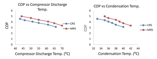
Figure 4: Comparison of COP with compressor discharge and condensation temperature
