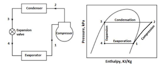
Figure 1: Schematic diagram of refrigeration system with enthalpy-pressure relation (Nasution et al., 2019)
