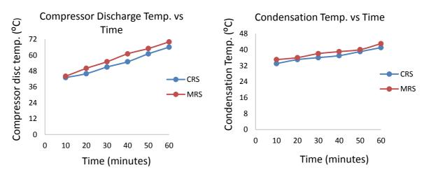
Figure 5: Comparison of compressor discharge and condensation temperature with time
