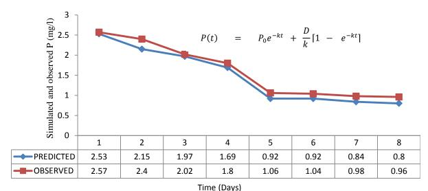
Figure 7: Simulated and observed variations for phosphorus removal in CW (P(t) = phosphorus concentration in wetland system (mg/l); Po = initial concentration of
