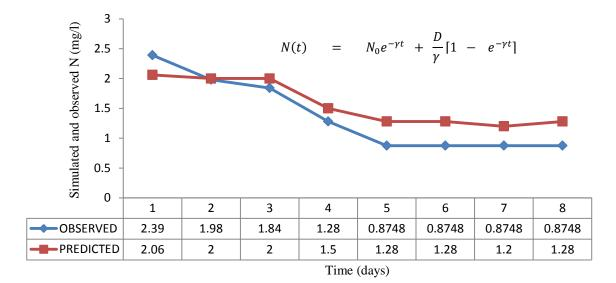
Figure 5: Simulated and observed variations for nitrogen removal in constructed wetland. (N(t) = nitrogen concentration in wetland system (mg/l); No = initial concentration of nitrogen (mg/l);  $\gamma$  = sum of nitrogen in wetland sinks (mg/l); D = rate of nitrogen input into the wetland (m³/day; t = wetland retention time (d))
