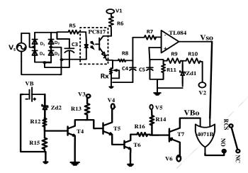
Figure 2: Codeless bi-controlled technique
