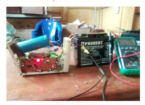
Figure 3: 11.7 VDC battery voltage from the digital meter with the proposed system
