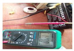
Figure 6: 14.40VDC battery voltage from digital meter with the proposed system
