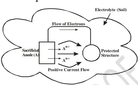
Figure 1. Schematic of Sacrificial Anode CP Method
