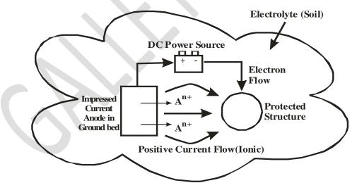
Figure 2. Schematic of Impressed Current Cathodic Protection Method (Michael et al., 2012)
