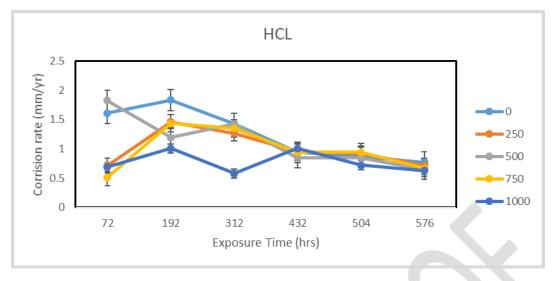
**Figure 11:** Variation of Corrosion Rate (mm/yr) against Exposure Time (hr) of low carbon steel in I M HCl at different concentration of leaves extracts on cathodic impress device
