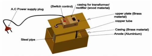
Figure 10. 3D model of Impressed Current electric device
