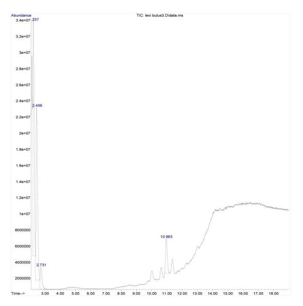
Figure 7: GC-MS fatty acid composition of neem biolubricant oil.
