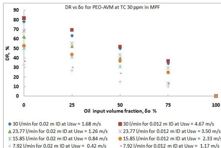
Figure 6: DR against oil input volume fraction at different flow rate (superficial velocity) and pipe diameter (0.012 and 0.02 m ID) in oil-water flow for PEO-AVM at total concentration of 30 ppm.
