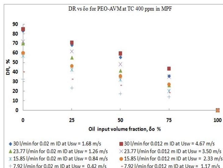
Figure 8: DR against oil input volume fraction at different flow rate (superficial velocity) and pipe diameter (0.012 and 0.02 m ID) in oil-water flow for PEO-AVM at total concentration of 400 ppm.
