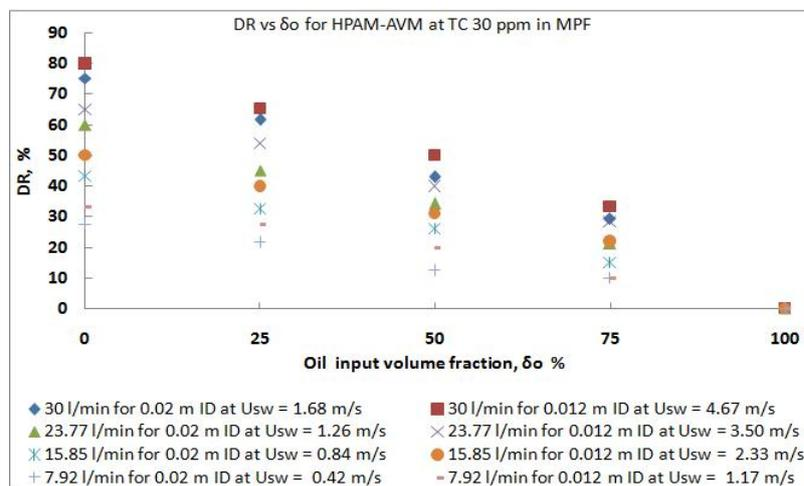
Figure 5: DR against oil input volume fraction at different flow rate (superficial velocity) and pipe diameter (0.012 and 0.02 m ID) in oil-water flow for HPAM-AVM at total concentration of 30 ppm.
