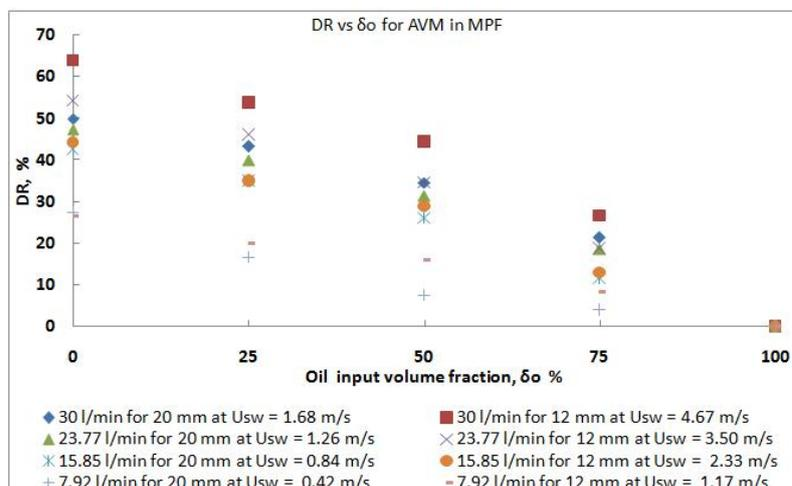
Figure 4: Effect of oil input volume fraction on drag reduction at different flow rate and pipe diameter (0.012 and 0.02 m ID) in oil-water flow for AVM.
