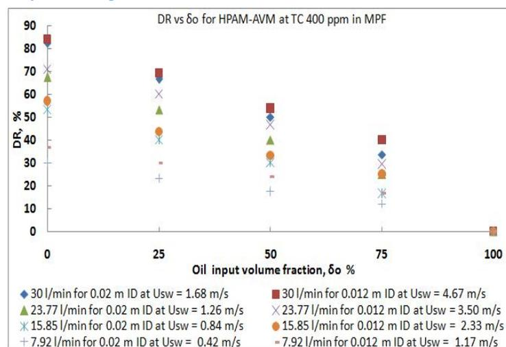
Figure 7: DR against oil input volume fraction at different flow rate (superficial velocity) and pipe diameter (0.012 and 0.02 m ID) in oil-water flow for HPAM-AVM at total concentration of 400 ppm.
