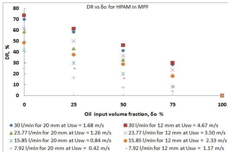
Figure 2: Effect of oil input volume fraction on drag reduction at different flow rate and pipe diameter (0.012 and 0.02 m ID) in oil-water flow for HPAM.
