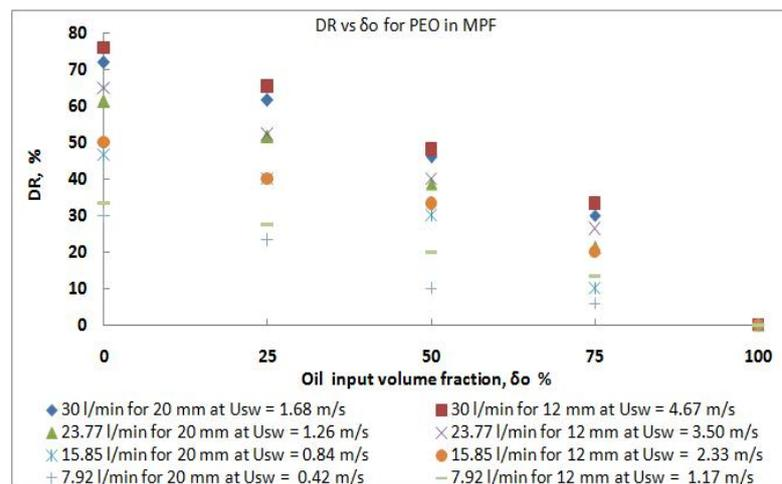
Figure 3: Effect of oil input volume fraction on drag reduction at different flow rate and pipe diameter (0.012 and 0.02 m ID) in oil-water flow for PEO.
