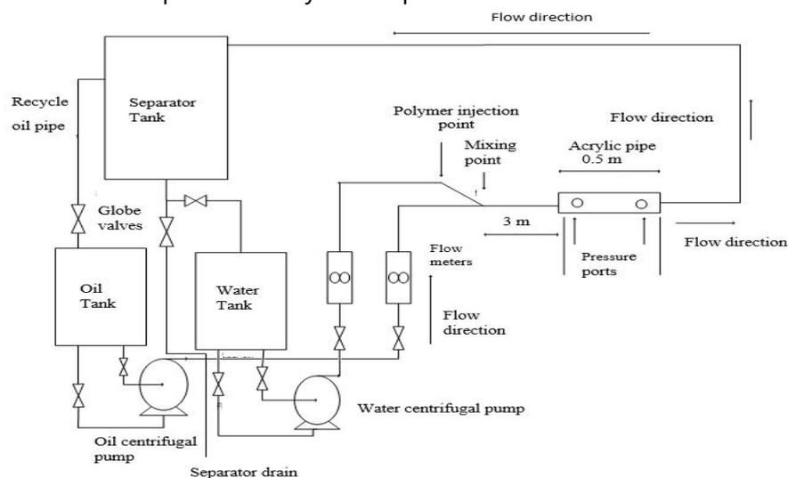
Figure 1: Schematics of experimental set-up of flow facility
