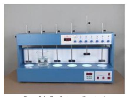
**Figure 5:** Jar Test Equipment (Flocculator)
