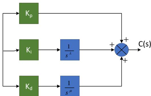
Figure 2. Block Diagram FOPID Controller
