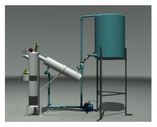
Figure 2: Isomeric View of the Distiller
