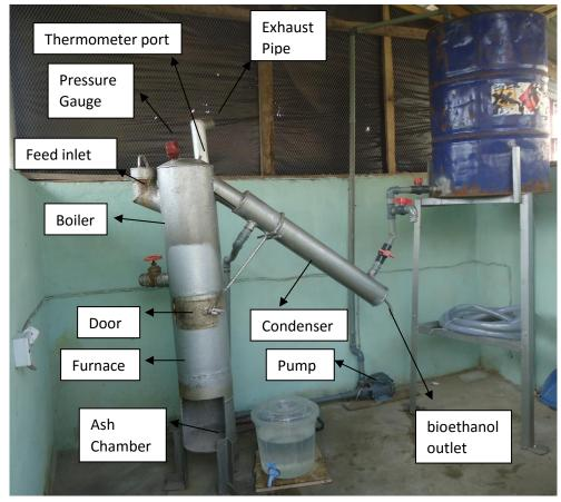
Figure 3: Pictorial View of the Fabricated Distiller
