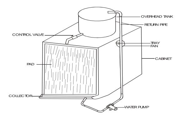
Figure 1: Schematic Diagram of the Evaporative Cooler
