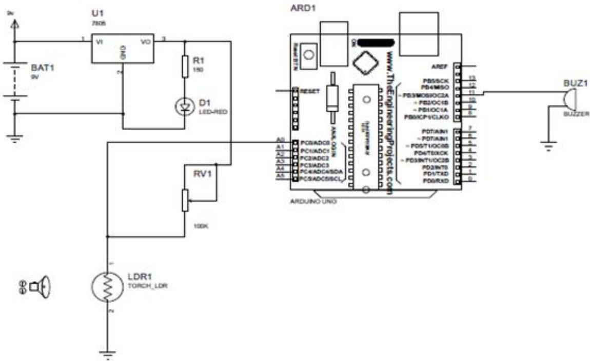
Figure 3: Circuit Diagram of an Arduino Based Alarm System
