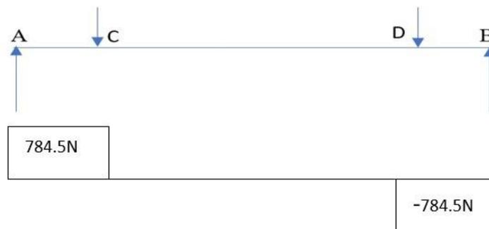
**Figure 5.** Shear Force Diagram
