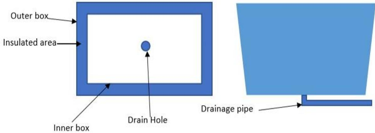
**Figure 1.** Illustration of the earlier design showing the drainage at the center of the box.
