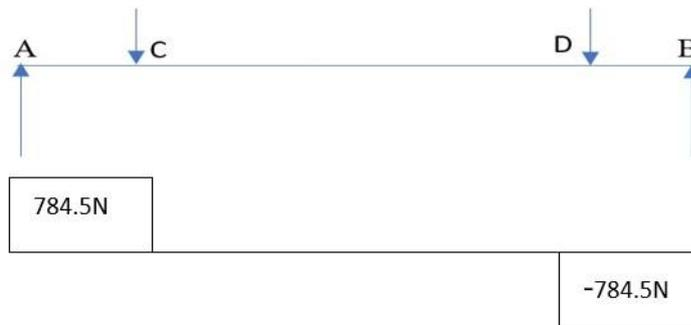
**Figure 5.** Shear Force Diagram
