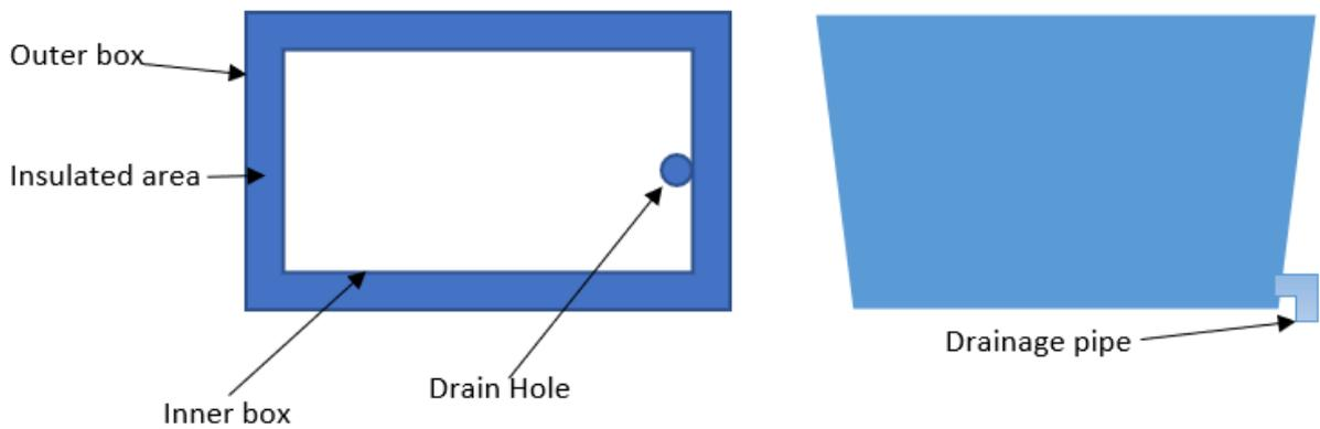
**Figure 2.** Illustration of the modified design showing the drainage at the center of the box.
