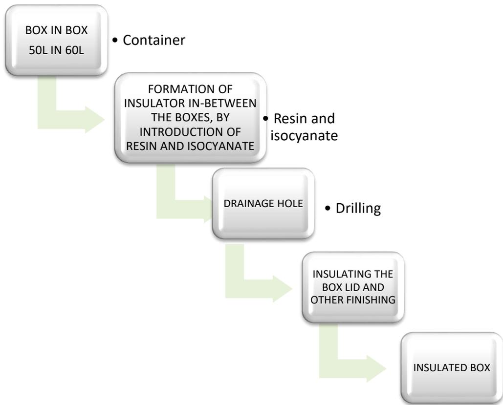
**Figure 3.** Flow chart showing process followed to producing an insulated box.
