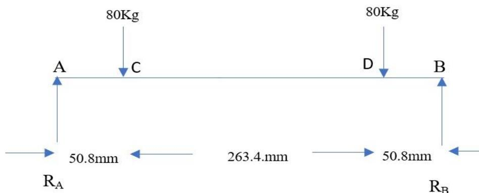
**Figure 4.** Load Diagram
