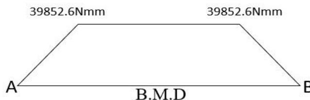
**Figure 6.** Bending Moment Diagram
