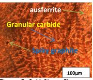
Figure 5: 0.41 % wt. Sb at 300 °C
