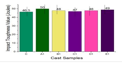
Figure 15: Variation of the Impact Toughness Values of the cast samples with wt%Sb for Ihour austempering time for an Austempering Temperature of 300°C
