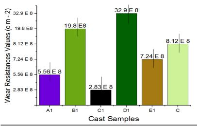
Figure 14a: Variation of the Wear Resistance Values of the cast samples with wt%Sb for 1 hour austempering time for an Austempering Temperature of 300°C
