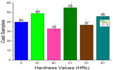
Figure 13: Variation of the Hardness values of the cast samples with wt%Sb for 1 hour austempering time for an Austempering Temperature of 300°C
