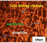
Figure 3: 0.24 % wt. Sb at 300 °C
