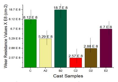
Figure 14b: Variation of the Wear Resistance Values of the cast samples with wt%Sb for 2 hours austempering time for an Austempering Temperature of 300°C
