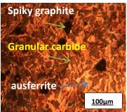
Figure 4: 0.34 % wt. Sb at 300 °C
