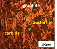
Figure 2: 0.12 %wt. Sb at 300 °C
