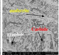
Figure 9: 0.24 % wt. Sb at 300 °C
