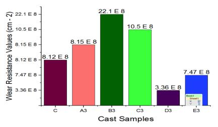
Figure 14c: Variation of the Wear Resistance Values of the cast samples with wt%Sb for 3 hours austempering time for an Austempering Temperature of 300°C
