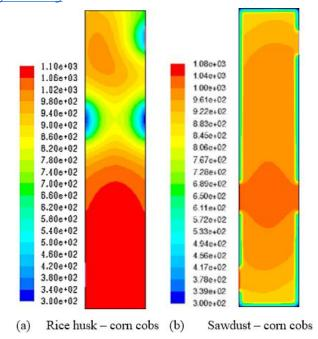
Figure 8: Contours of temperature with variations in fuel mixtures
