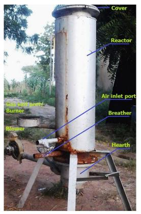
Figure 1: Downdraft Gasifier facility developed by Abubakar (2013)
