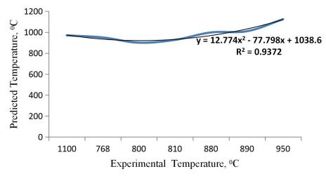
Figure 4: Experimental and CFD Predicted results validation
