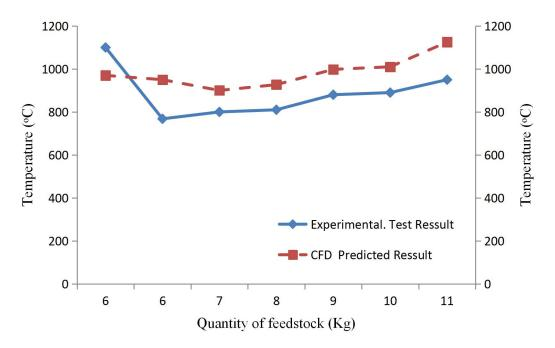
Figure 3: Experimental and Computational results for rice husk and sawdust
