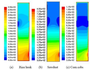
Figure 7: Contours of temperature with variations in fuel types
