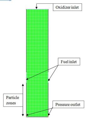
Figure 2: A 2-D Meshed Model of the gasifier.
