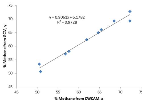
**Figure 6:** Correlation between the GCM and CWCAM results of % methane determination
