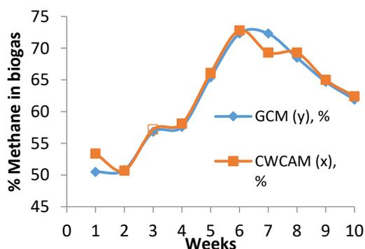
**Figure 5:** Comparisons between the GCM and CWCAM results for % methane determination.
