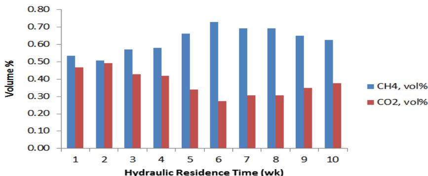
**Figure 4:** Methane and carbon dioxide contents in produced biogas (analysis based on CWCAM)
