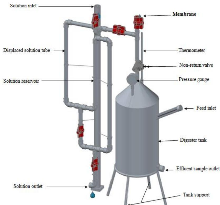
**Figure 1:** 15 l capacity digester system
