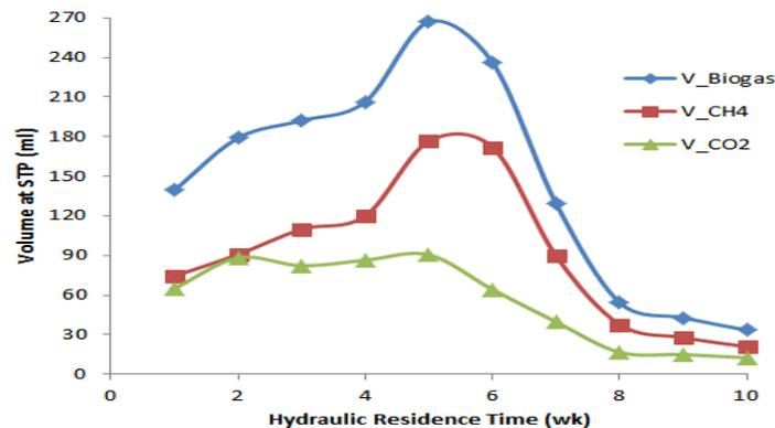
**Figure 3:** Biogas, methane and carbon dioxide production profiles based on CWCAM
