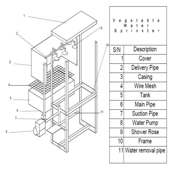
Figure 2: Vegetable Moisturizer Assembly (Vegetable Water Sprinkler)
