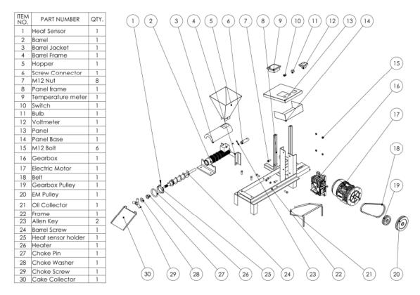
Figure 3: Exploded drawing of a motorized tiger nut oil extracting machine
