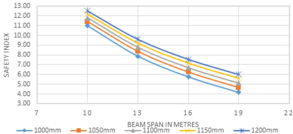
**Figure 4:** Flexural safety index Vs Beam span for various beam depth for 30 N/mm<sup>2</sup> characteristic strength of concrete
