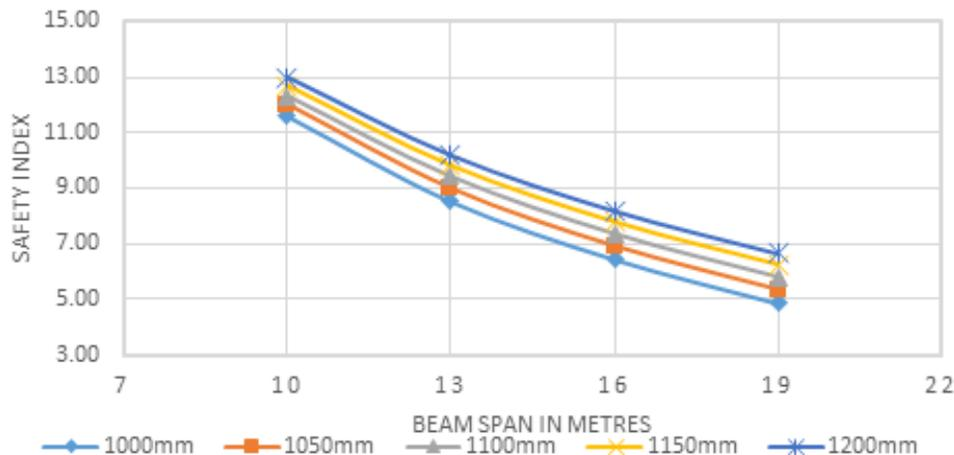
**Figure 5:** Flexural safety index Vs Beam span for various beam depth for 35 N/mm<sup>2</sup> characteristic strength of concrete
