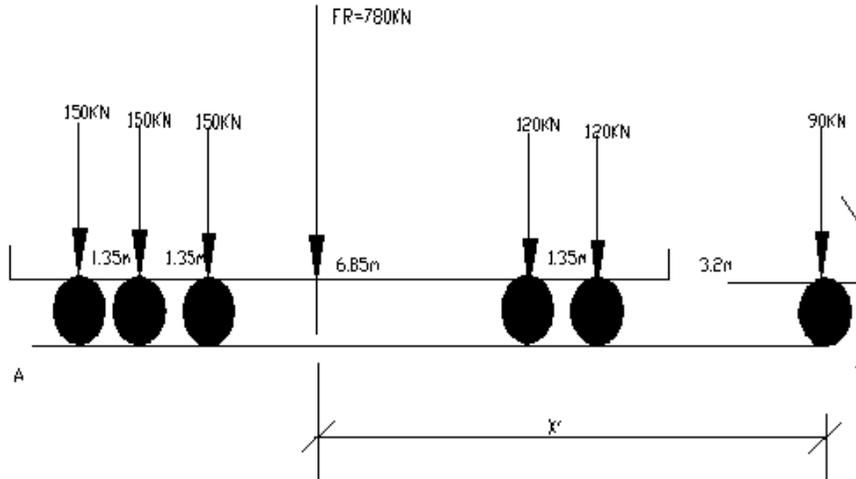
**Figure I:** Load Distribution on 6-Axles (Sinotruck) according to Eurocode
