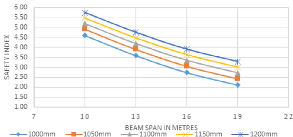
**Figure 7:** Flexural safety index Vs Beam span for various beam depth for 50 N/mm<sup>2</sup> characteristic strength of concrete
