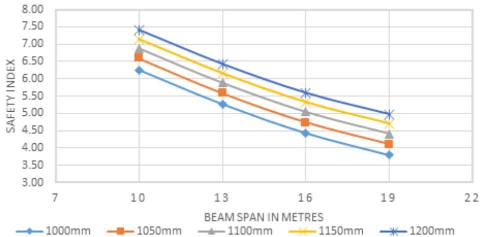
**Figure 10:** Shear safety index Vs Beam span for various beam depth for 40 N/mm<sup>2</sup> characteristic strength of concrete
