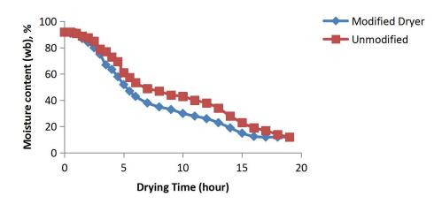
Figure 4: Variation of moisture content with time in the dryer
