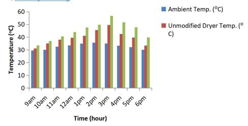
Figure 3: Variation of temperature inside and outside the dryer as a function of time in the second day
