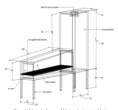
Figure 1: Schematic diagram of fabricated solar vegetable dryer
