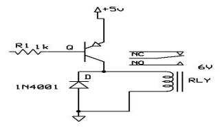
Figure 7: Circuit of Transistor
