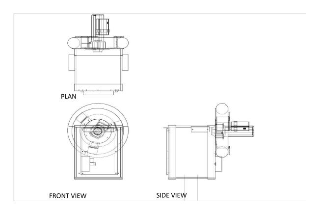
Figure 3: Orthographic Projection of Airbag Mechanism
