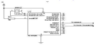
Figure 5: Circuit Diagram of Controller Unit.
