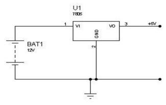
Figure 3: circuit diagram of the power.
