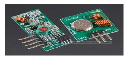
Figure 6: The Pictorial View of RfTx and Rx.
