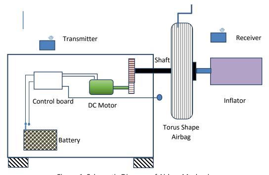
Figure 1: Schematic Diagram of Airbag Mechanism
