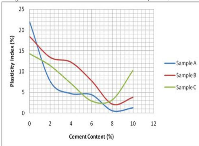
Figure 3: Variation in plasticity indices for soil samples A, B and C
