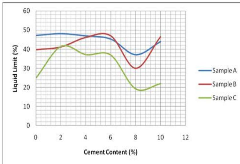
Figure 1: Liquid limit variations for soil samples A, B and C
