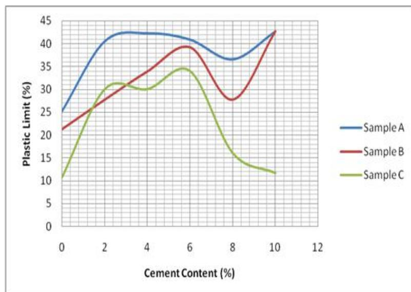
Figure 2: Plastic limit variations for soil samples A, B and C
