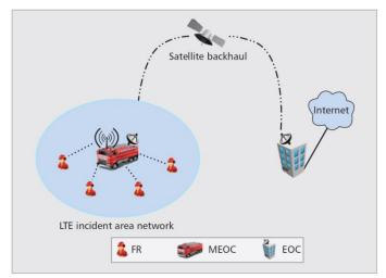
Figure 10: LTE System with integrated Satellite Backhaul (Casoni et al., 2015)
