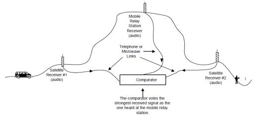
Figure 7: Satellite and Mobile relay system (Kathy and Hart, 2003).
