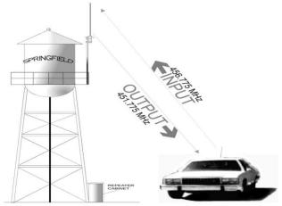
Figure 6: Two-way repeater stations (Wiki, 2016a)
