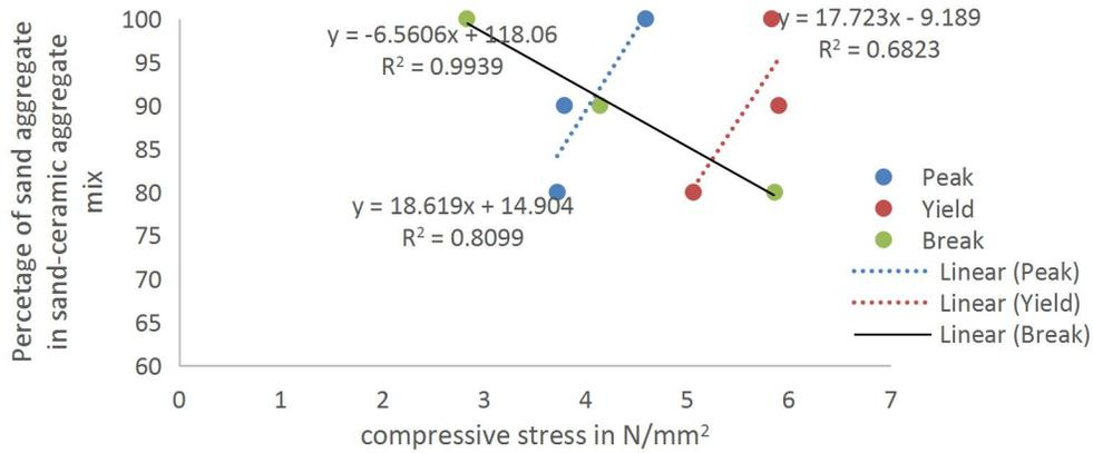
Figure 13: Aggregate mix ratio and compressive stress nexus
