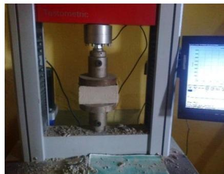
Figure 5: Masonry unit under compressive test
