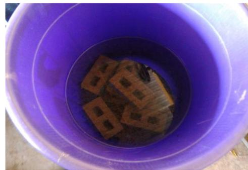
Figure 4: Hollow masonry unit under curing
