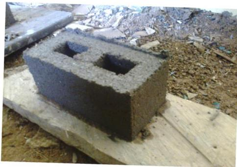
Figure 3: Freshly moulded hollow block
