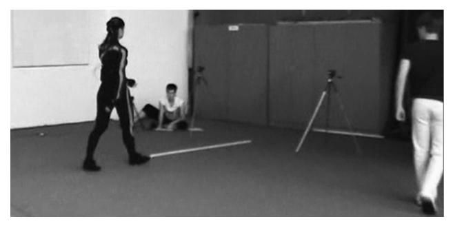
*Fig 1.* Measurement set-up: (i) a subject in the MOV dress that wirelessly transfers the data to the computer which was operated by the first measurer, (ii) the sitting measurer was noting down the time acquired by the photocells and made additional precise measurements of the last remaining step using the measurement tape, (iii) the third measurer was only estimating the length of the last step and measuring the time with the manual stop-watch.
