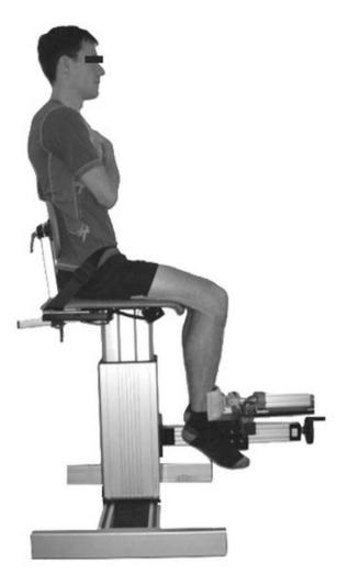
Fig 1. Measuring system "SeBit knee" for the detection of Adaptive Force (AF) of the quadriceps femoris muscle.
