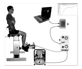
Fig. 1 Measuring system to determine the Adaptive Force
