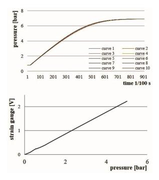
*Fig 4.* Above: Diagram of ten pressure curves measured in a row (sampling rate 100 Hz). Below: Scatter diagram between rises of the strain gauge and of the pressure signal.
