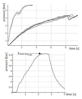
*Fig.* 3. Pressure curves [bar] measured by the system SeBit knee. Above: Five trials of measuring the AF of one subject during slow (black) and rapid (grey) pressure increase. The data are filtered with butterworth filter (filter degree 10, cut-off frequency 3 Hz). Bottom: One trial of maximum concentric-isometric force Fcon-iso<sub>max</sub>.
