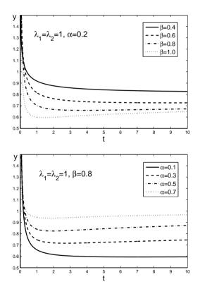
Fig. 3. Time profiles of the pressure gradient for  $\alpha < \beta$ , A = 1 and  $\lambda_1 = \lambda_2 = 1$ .
