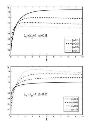
Fig. 4. Time profiles of the pressure gradient for  $\alpha > \beta$ , A = 1 and  $\lambda_1 = \lambda_2 = 1$ .
