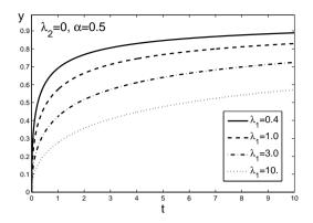
Fig. 2. Time profile of the pressure gradient for A = 1,  $\lambda_2 = 0$ ,  $\alpha = 0.5$  and various values of  $\lambda_1$ .
