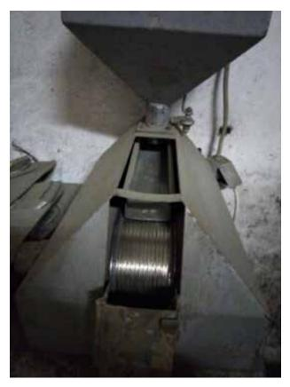
Fig. 1. Laboratory magnetic separator German manufacturer Emceka Gompper
